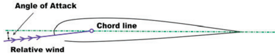
Fig. 1 | If the angle of attack is positive, lift is created. If the angle of attack increases, drag increases, and we slow down on both axes (horizontal and vertical) until a new equilibrium is reached.
